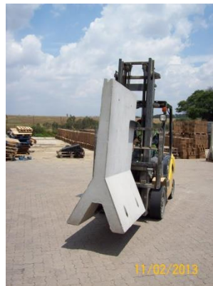
Forklift using carrier attachment
